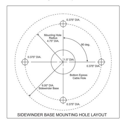
The base of the Sidewinder SW720-H.264-HD camera has four ½-20 screw holes that are equally spaced, 90 degrees apart, on a 4.75" diameter circle, as shown in figure 2 (Note that 24VAC versions of the Sidewinder camera will have 5/16" mounting screws). If mounting screws other than those provided with the camera are used, the length of the mounting screws should be selected so that the screws penetrate no more than 0.75 inches into the base.
